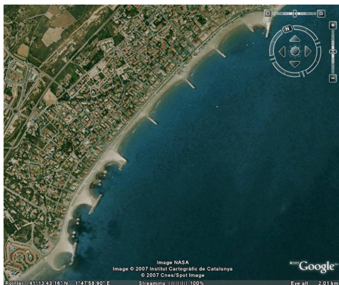
Fig. 15. Coastal protection by various hard structures at beach of Sitges, south of Barcelona, Spain.
